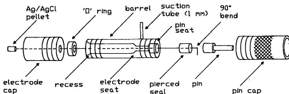
Five spare 'O' rings and one spare pierced seal are provided with each holder. Additional 'O' rings, pierced seals, pins and Ag/AgCl pellet assemblies can be purchased from Axon Instruments.
