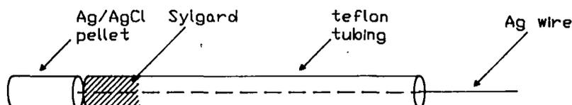
It is not practical to make a pellet small enough to fit inside the shaft of the narrow glass electrodes used in the and HL-2-12 holders, therefore these holders are supplied with a piece of 0.25 mm silver wire. It is up to
