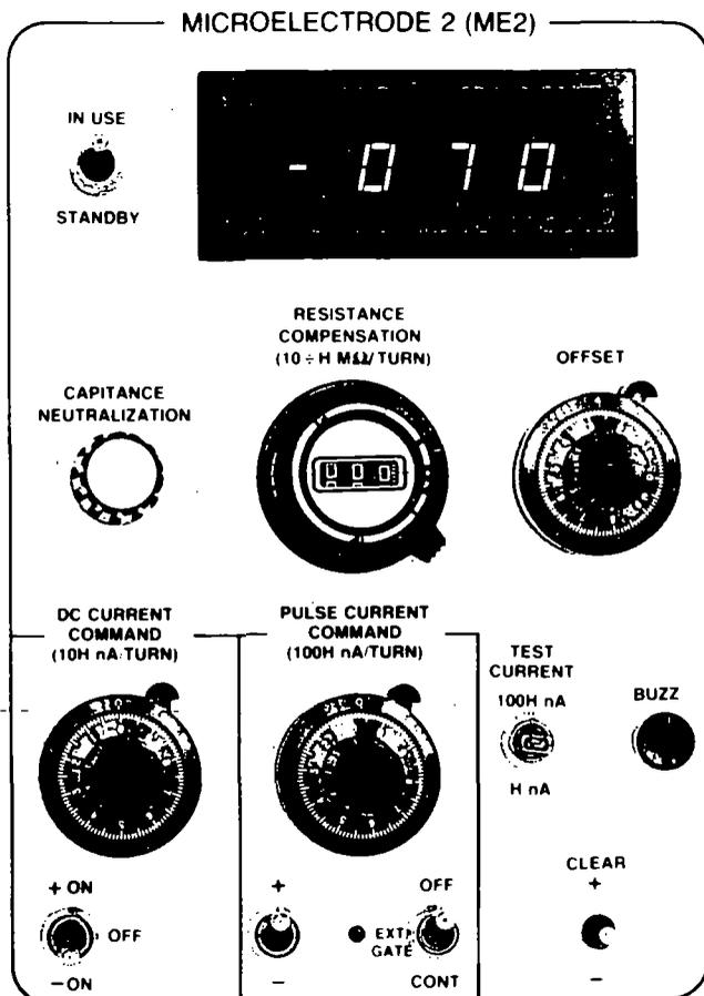
During current passing the voltage drop across the microelectrode can be eliminated from the electrode voltage by setting the **Resistance Compensation** control (also known as Bridge Balance control). At this setting the microelectrode resistance can be read from the dial. Alternatively, the microelectrode resistance can be read on the digital panel meter by using the **Test** switch.
